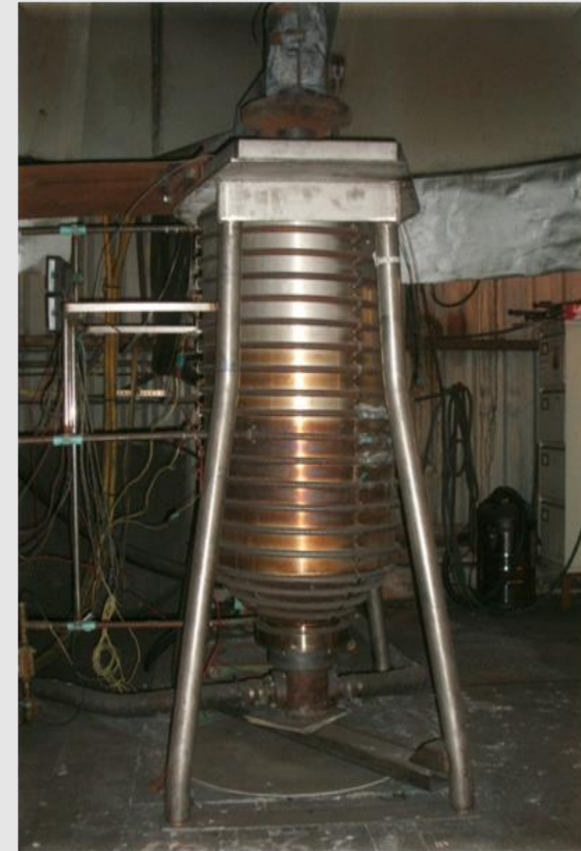
The picture shows the 100 kW with a calcination furnace installed
